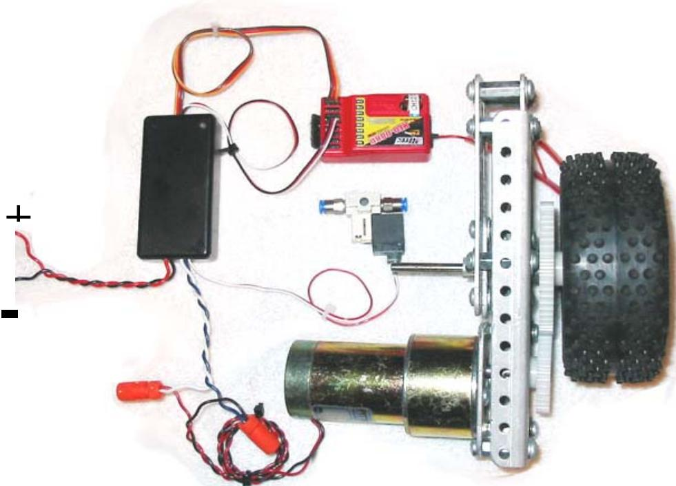
The picture above illustrates how to connect the GEARS II or III Combination Controller to the RC receiver, Gear Head Motor, Pneumatic Solenoid Valve and the Battery (Not Shown).
