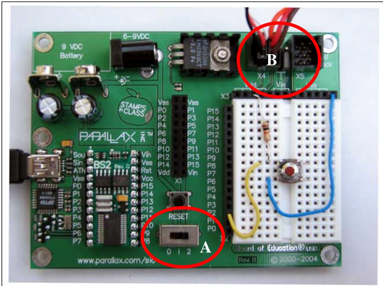
This is the wiring that allows the example code to operate the two channels of a GEARS II or III Speed Controller. The circuit on the breadboard is the same circuit shown in the schematic on page 4.
